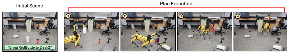
Fig. 1: Demonstration of our approach, CoReLIN, deployed on the Boston Dynamics Spot robot. CoReLIN first observes the initial scene and determines the presence of task-relevant objects (e.g., Bottle and Desk) alongside environmental clutter. Based on the observations, current task progress, and cost-benefit analysis, our approach determines the best course of action (“Move PaperTowelRoll to BlackBox”, “Move RedBottle to Desk2”). CoReLIN first optimizes the environment by moving the clutter (the paper towel roll) to a carefully chosen out-of-the-way spot (the black box). It can then place the red bottle on the desk.
